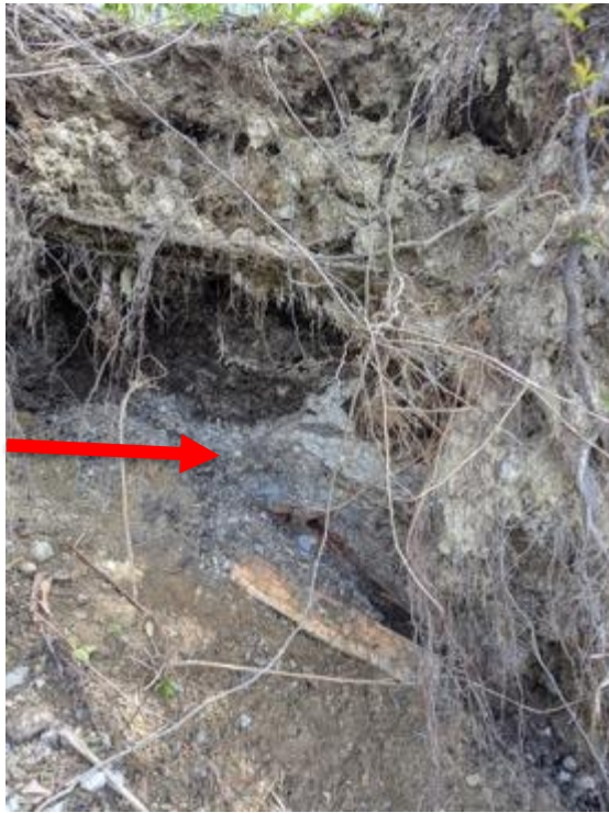
Field Sampling Photo 16: View of sample GAC-Sed-G (red arrow). Material is grayish white and powdery. Low pH (5.09), aluminum (190 mg/kg) and sulfur (64,000 mg/kg) present.
