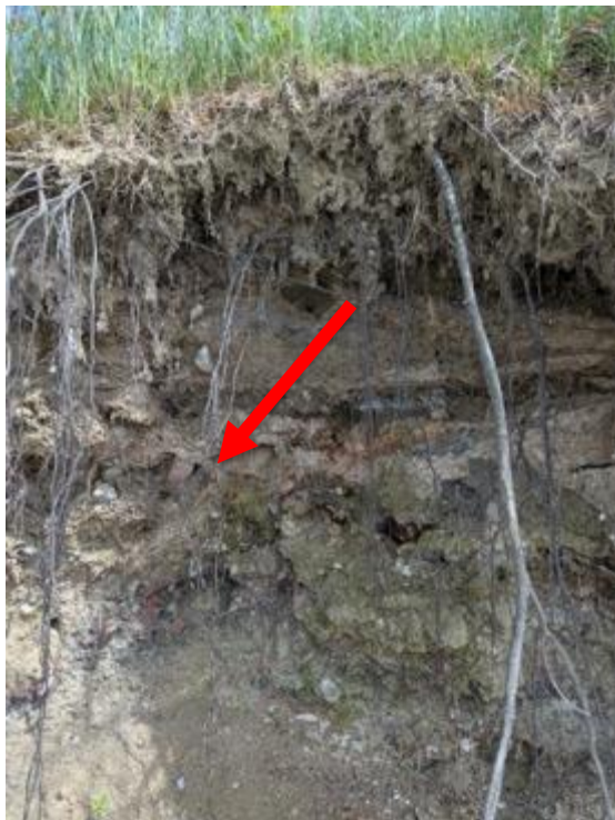
Field Sampling Photo 19: View of sample GAC-Sed-I (red arrow), collected ~2' below top of bluff. Low pH (4.67), and aluminum (19,000 mg/kg) and sulfur (120,000 mg/kg) detected.
