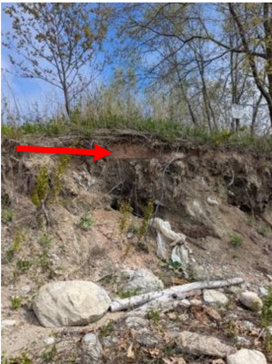
Field Sampling Photos 17 and 18: View of sample GAC-Sed-H (red arrow). Distinct layer within exposed bluff of reddish material. Low pH (4.81), and aluminum (100,000 mg/kg), sulfur (390 mg/kg) and mercury (0.39 mg/kg) detected.
