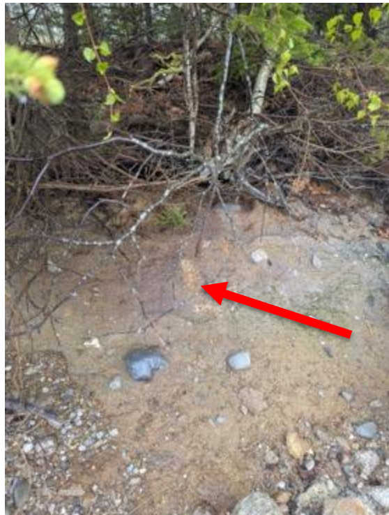
Field Sampling Photos 14 and 15: View of sediment sample GAC-Sed-F (red arrow). Material is hard, crumbly fill, does not appear to be natural sediment. Extremely low pH (2.67), and aluminum (2,200 mg/kg) and sulfur (6,700 mg/kg) detected.
