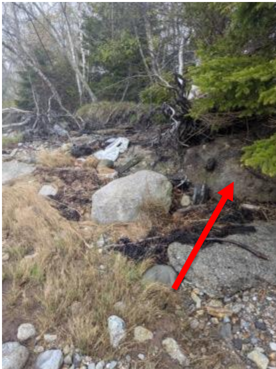
Field Sampling Photos 14 and 15: View of sediment sample GAC-Sed-F (red arrow). Material is hard, crumbly fill, does not appear to be natural sediment. Extremely low pH (2.67), and aluminum (2,200 mg/kg) and sulfur (6,700 mg/kg) detected.
