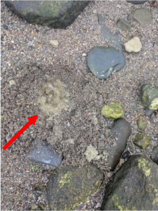
Field Sampling Photos 9 and 10: View of sample GAC-Sed-C (red arrow), sediment collected from intertidal area, approximately 6" below surface and 10 yards south of the pipeline. Aluminum (20,000 mg/kg) detected.
