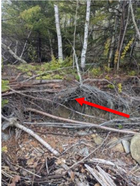
Field Sampling Photo 13: View of sediment sample GAC-Sed-E (red arrow) collected from exposed bluff, ~1' below top of bluff. Extremely low pH (4.16), and aluminum (3,100 mg/kg) and sulfur (520 mg/kg) detected.
