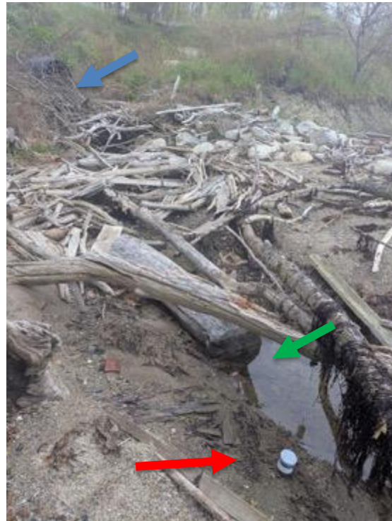
Field Sampling Photos 1 and 2: View of sediment sample GAC-Sed-A (red arrow) and water samples GAC-Water-A (blue arrow) and GAC-Water-B (green arrow). Low levels of sulfur and aluminum detected in water, and aluminum (6,700 mg/kg) in soil.
