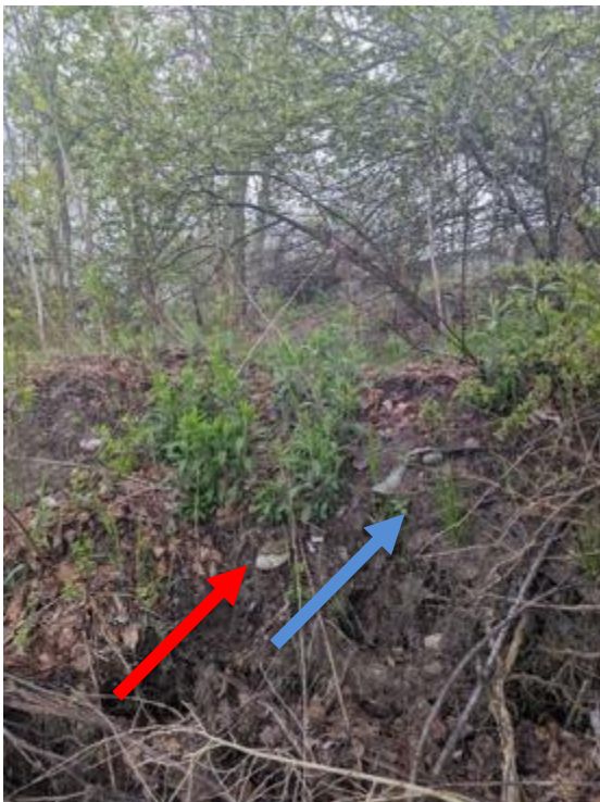
Field Sampling Photos 3 and 4: View of sediment sample GAC-Sed-B (red arrow) collected from exposed bluff, aluminum (19,000 mg/kg), sulfur (1,200 mg/kg) and mercury (0.12 mg/kg) detected. Building material sample GAC-BM-A (blue arrow) contained lead (9.6 mg/kg).
