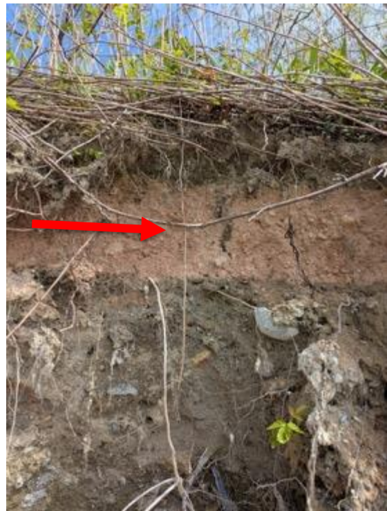
Field Sampling Photos 17 and 18: View of sample GAC-Sed-H (red arrow). Distinct layer within exposed bluff of reddish material. Low pH (4.81), and aluminum (100,000 mg/kg), sulfur (390 mg/kg) and mercury (0.39 mg/kg) detected.
