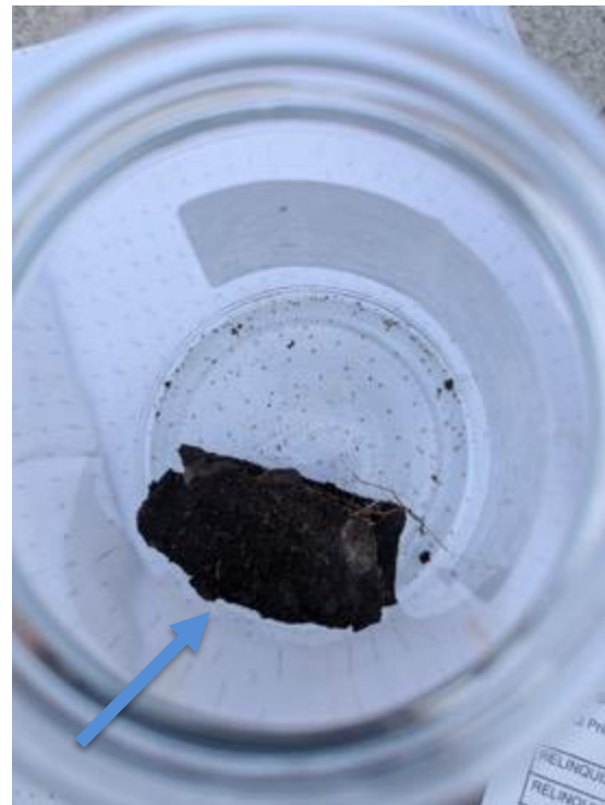
Field Sampling Photos 3 and 4: View of sediment sample GAC-Sed-B (red arrow) collected from exposed bluff, aluminum (19,000 mg/kg), sulfur (1,200 mg/kg) and mercury (0.12 mg/kg) detected. Building material sample GAC-BM-A (blue arrow) contained lead (9.6 mg/kg).
