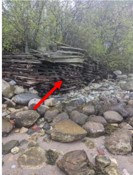
Field Sampling Photos 5 and 6: View of building material sample GAC-BM-B, black, tar-like coating on wood. This coating is located throughout this wood debris pile area.
