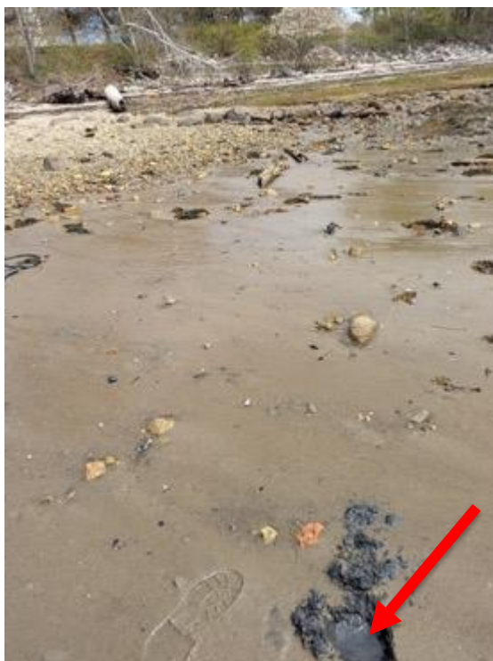
Field Sampling Photo 20: View of sample GAC-Sed-J (red arrow), collected from intertidal area, approximately 6" below surface. Aluminum (10,000 mg/kg), sulfur (3,500 mg/kg), mercury (0.14 mg/kg)
