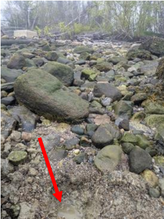
Field Sampling Photos 11 and 12: View of sample GAC-Sed-D (red arrow), sediment collected from ~6" below surface of intertidal area. Aluminum (8,700 mg/kg) and sulfur (120 mg/kg) detected.
