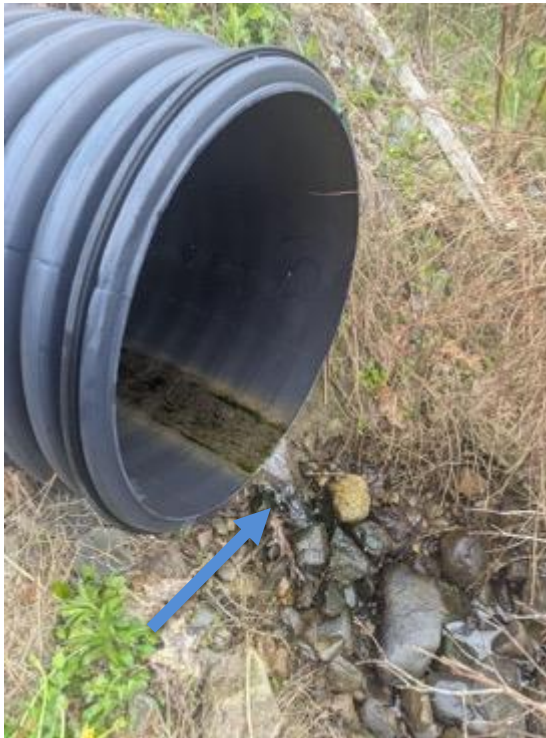
Field Sampling Photos 1 and 2: View of sediment sample GAC-Sed-A (red arrow) and water samples GAC-Water-A (blue arrow) and GAC-Water-B (green arrow). Low levels of sulfur and aluminum detected in water, and aluminum (6,700 mg/kg) in soil.
